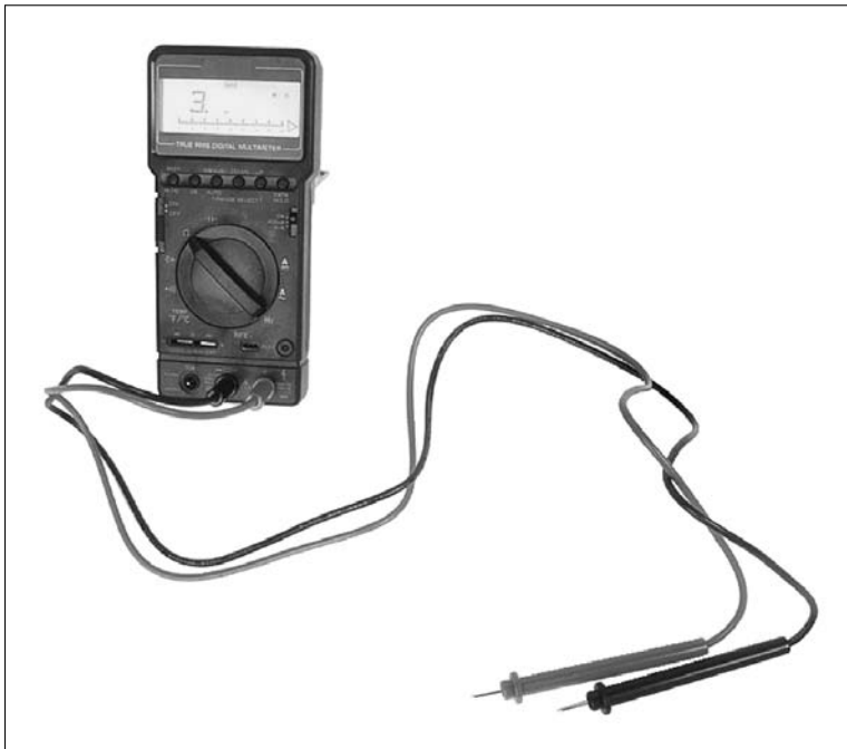
Figure 12-1: Multimeters measure voltage, resistance, current and continuity.
