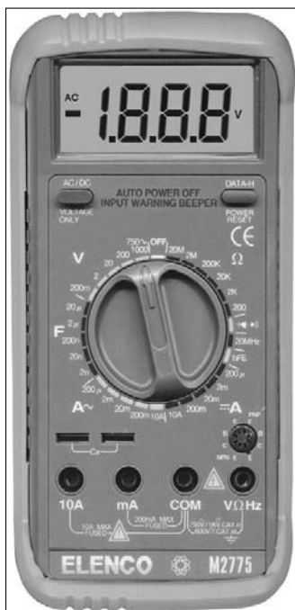
Figure 9-2: Multimeters measure voltages, resistance and current.
