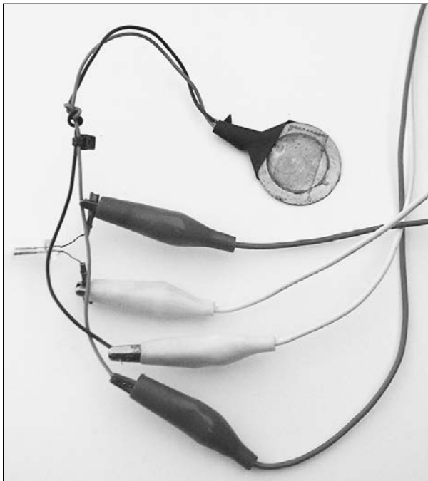
Figure 14-4: Connect the disc and neon lamp using croco- dile clips.
