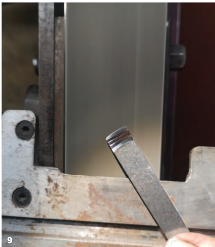
7 Rough grinding the bevels, showing the sweep needed to reshape them 8 Bevels formed at 60 grit. Notice how the curves of the front and back of the bevel match 9 Bevel marked up and ready to grind on a finer belt 10 Stropped with no obvious micro bevel
