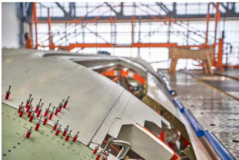
The upper frame shell of an A330-200P2F EPW
