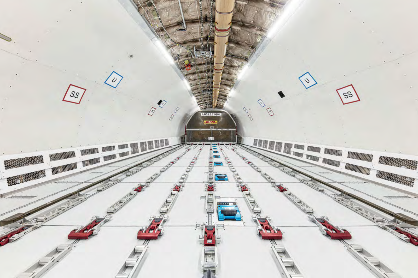
A rare glimpse inside a P2F once the engineering work is complete and the jet is ready for its new role as a freighter EFW
