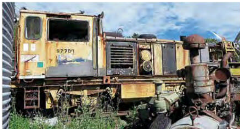
Shunting loco No. 97701 is the only example of its type, being a 4wDE conversion from the power unit of a Matisa ballast cleaner. It is seen in a secure yard in East Sussex in August. ANTHONY BARTON
