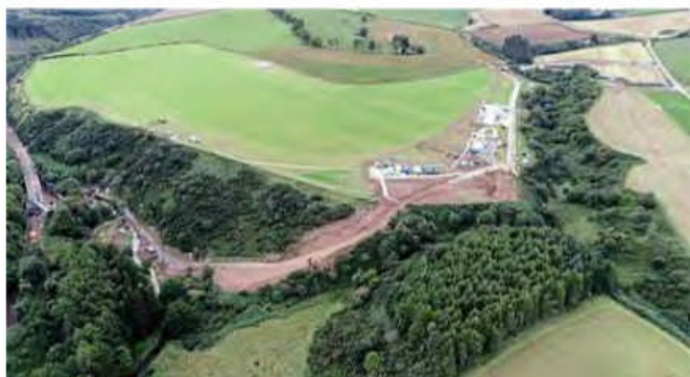
Left: An aerial view showing the new access road and work compound which have been built to recover the HST in the Carmont derailment. The line is on the extreme left, and the nearest road on the extreme right. NETWORK RAIL
