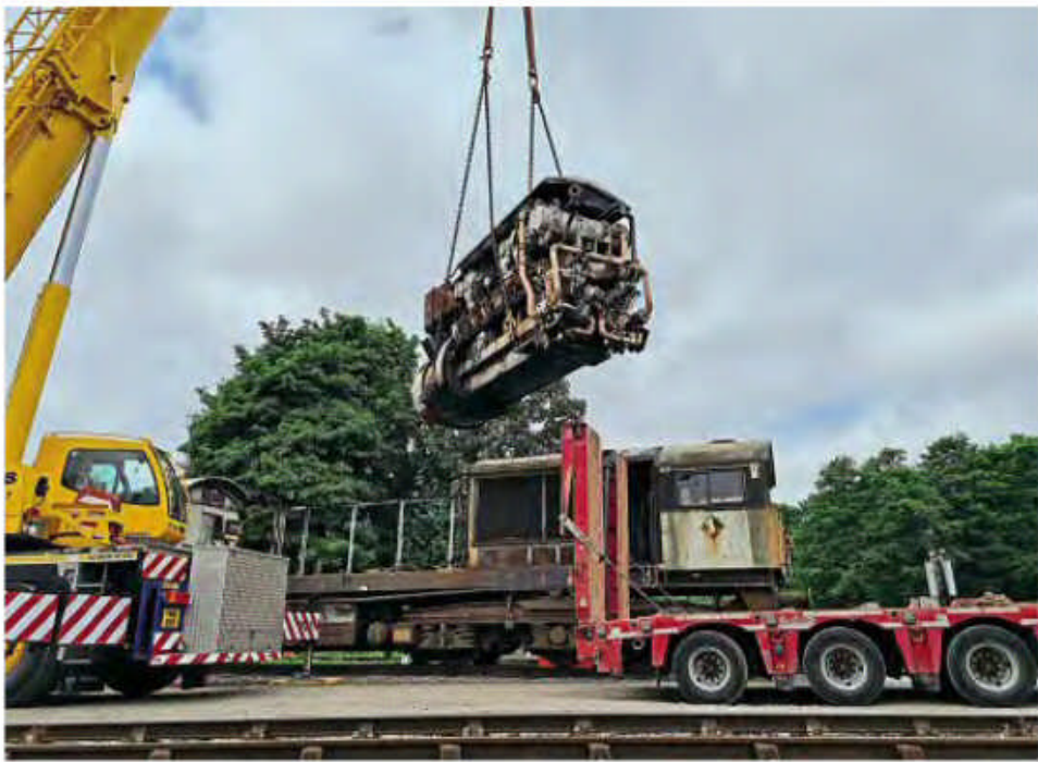
The engine, silencer and alternator are removed from No. 58022 at Peak Rail, Rowsley, on August 11, prior to moving the rest of the loco to the Ecclesbourne Valley Railway. IDRS
