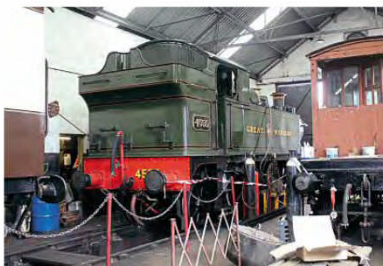
No. 4555 stands in the back of the shed at Cranmore on August 31 with various equipment attached for examination of the firebox. PETER NICHOLSON
