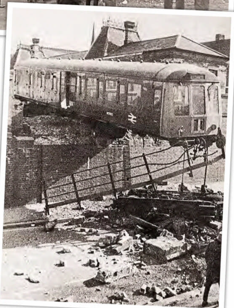
There have been a few accidents in and around Stourbridge, such as the shunting incident at Amblecote in 1905 (above) and another spectacular one on April 2, 1977, when Class 122 No. 55012 failed to stop at Stourbridge Town after a brake failure, went through the buffer stops and a retaining wall, leaving it suspended over Foster Street.
